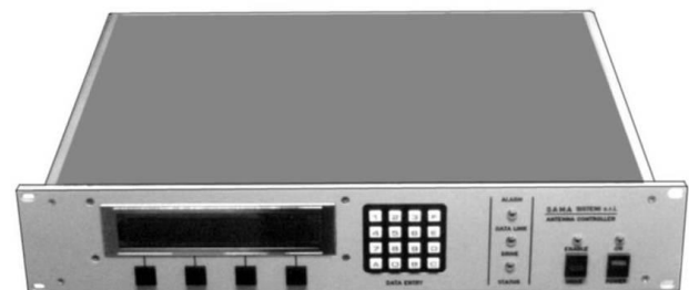
Antenna Control Unit (ACU): front view
